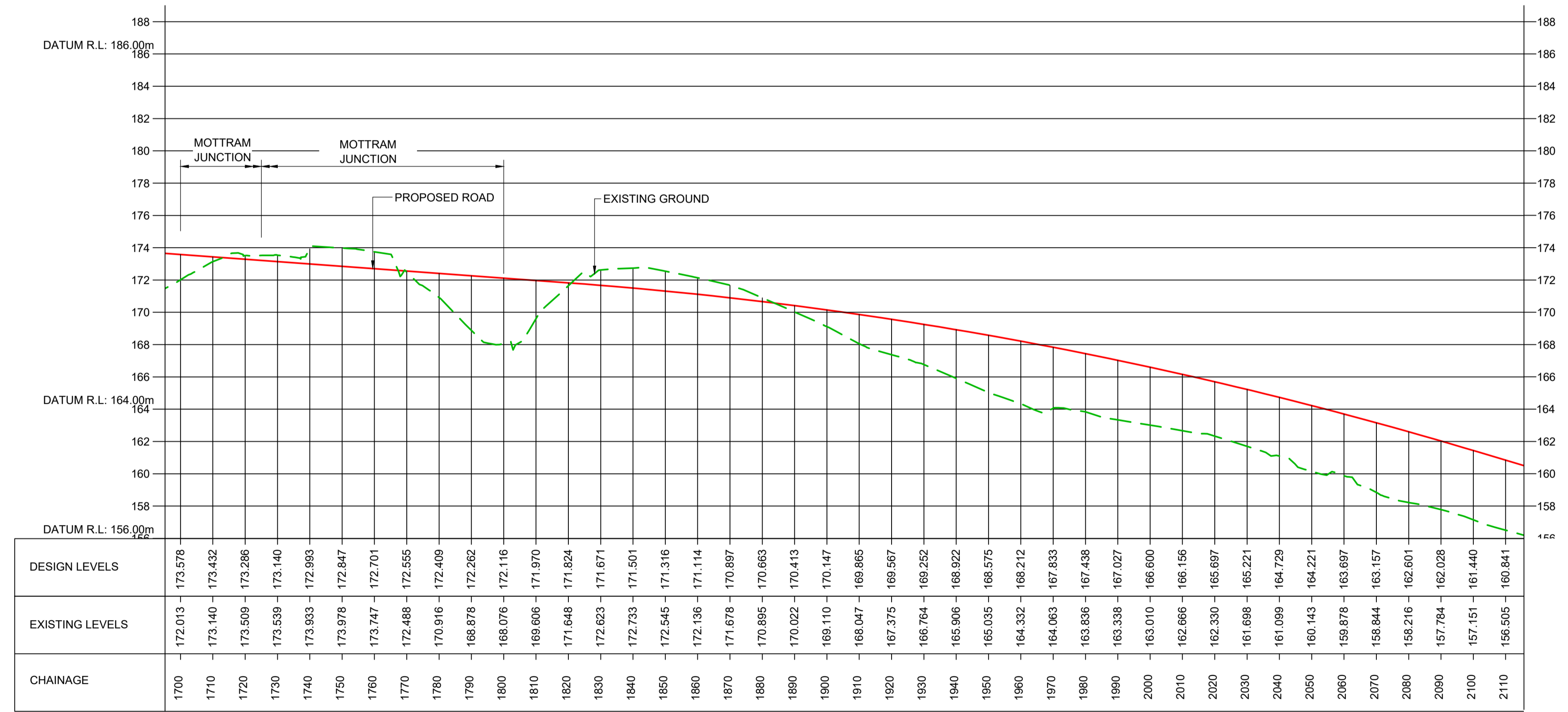
LONGITUDINAL SECTION - A57 MAINLINE ALIGNMENT
