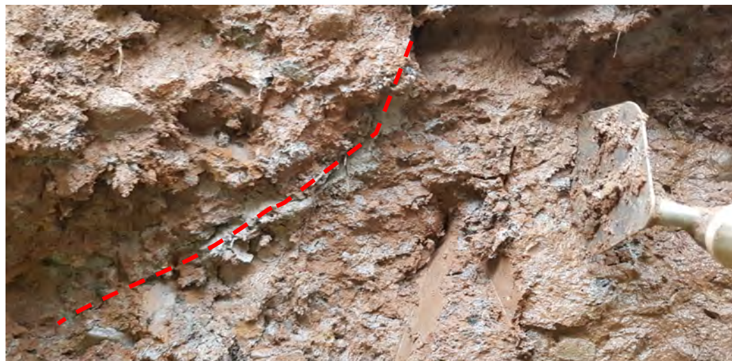
Photo 06: Possible 60 shallowing to 45 degree slip surface identified in Face B
