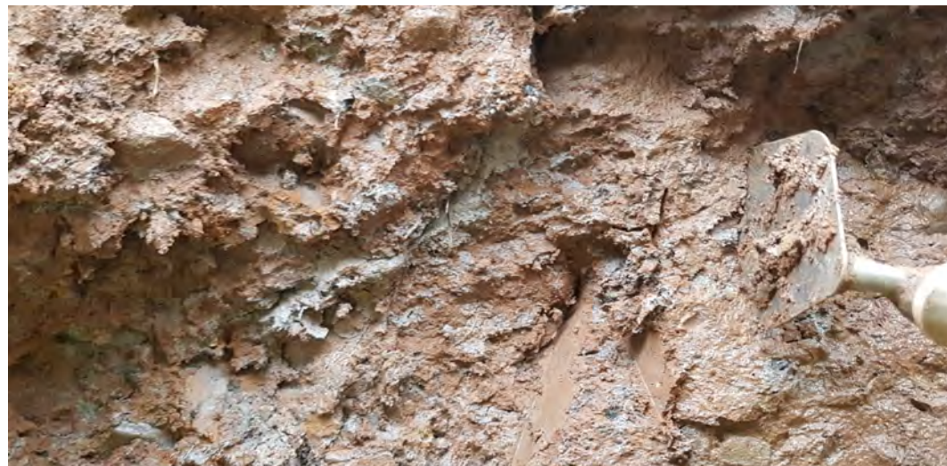
Photo 06: Possible 60 shallowing to 45 degree slip surface identified in Face B
